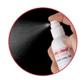
The surface tension is determined by spraying test ink onto the surfaces to be assessed.
